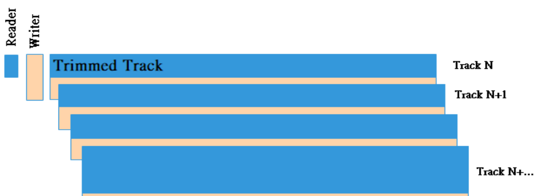
Figure 1. Overlapping Tracks in SMR Technology
