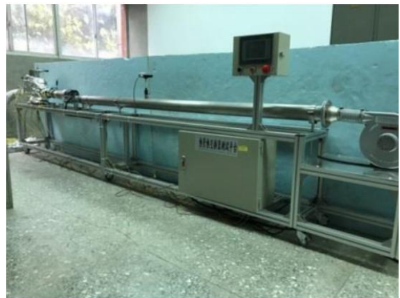
Fig. 2.5 Picture of the heat pipe heat exchanger
